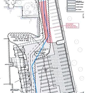
2. Please also see the red outline for limits of pavement replacement to be sure no slivers of pavement remain. Uniform pavement repair/replacement shall be done when possible (See General Note No. 4).
